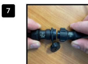
Attach the sensor cable to the Agbot. Make sure the white dots on both the sensor cable connector and the Agbot connector line up – do not force it.
