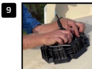
Secure the Agbot into the mounting bracket. Simply push it in until it clicks into place.
