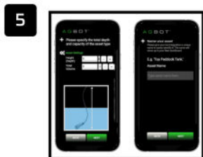
In the Agbot app, select Add Device and select your asset type, sensor type and length, insert the asset dimensions for Height (Depth) in Metres and Total Volume in Litres.
