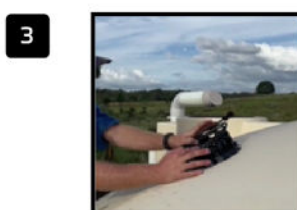
Lower the sensor probe to the bottom of your tank. Make sure it is definitely on the bottom. Secure the remaining cable in the cable bracket.
